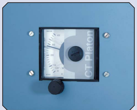
Purge Model APV Mounted in control panel
